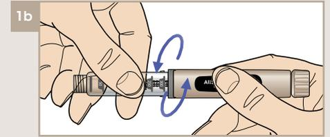
1b Unscrew the cartridge holder from the pen body.
